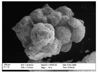
Figure 4. Low magnification scanning electron microscopy image of mamillary precipitate of calcite.
