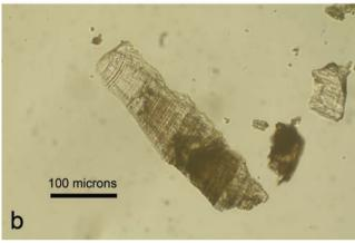
Figure 5. a) Scrapings of the phosphatic precipitate mounted in oil and viewed using plane-polarised light microscopy; b) a calcite crystal from the mamillary precipitate mounted in oil and viewed using plane-polarised light microscopy. Note the growth bands perpendicular to the elongated crystal (both images taken in picture processing language).
