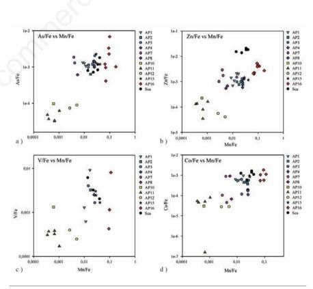
Figure 5. Bivariate plots of a) As/Fe, b) Zn/Fe, c) V/Fe, and d) Co/Fe ratios compared to Mn/Fe ratio in the pigments of the Abri Pataud analysed by PIXE. The sample AP13, which does not contain any Mn, was not plotted on these graphs.
