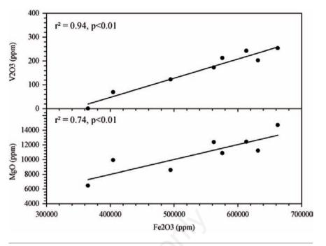
Figure 4. Concentration of V and Mg oxides (ppm) as a function of iron oxide concentration for samples AP11 and AP12.
