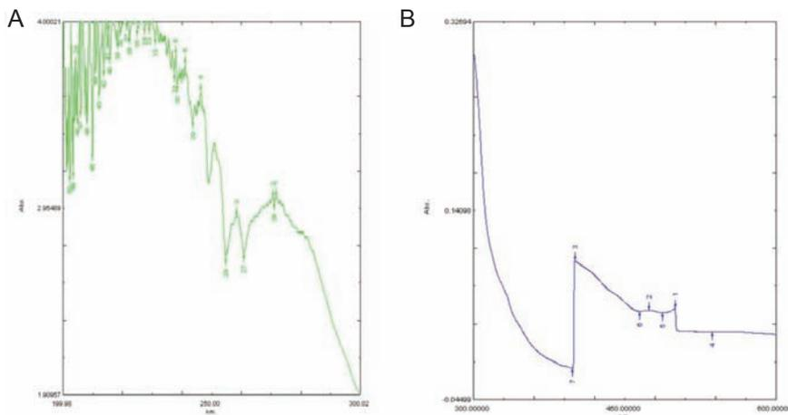
Figure 2. UV-Vis absorption spectrum of *Ceiba pentandra* seed oil. A) Absorption spectra from 200 nm to 300 nm; B) Absorption spectra from 300 nm to 600 nm.
