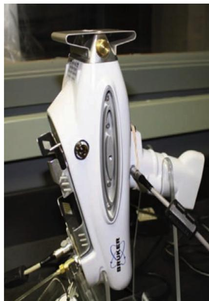
Figure 2. Bruker AXS tracer III-V handheld X-ray fluorescence spectrometer (Bruker, Billerica, MA, USA).
