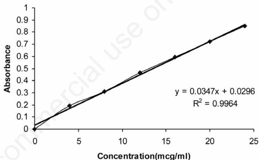
Figure 1. Calibration curve of Aspirin in methanol: water (1:9) system.
