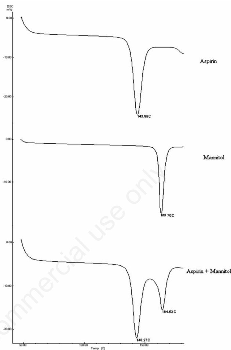
Figure 2. DSC Thermograms of ASP, Mannitol and ASP with Mannitol.
