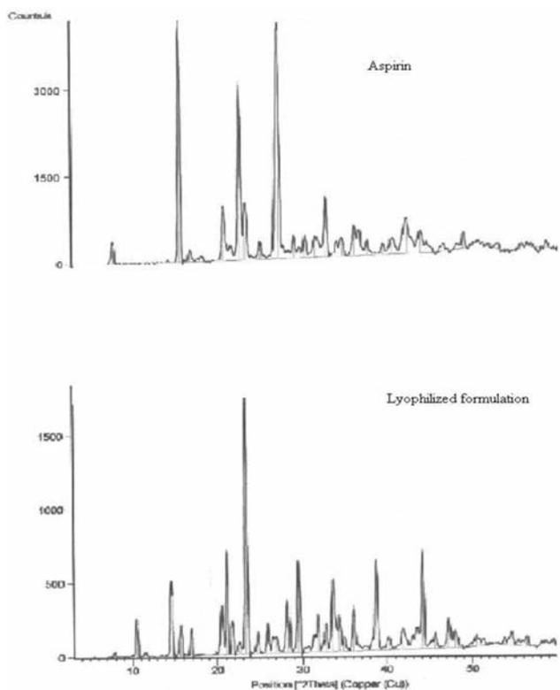
Figure 3. X-ray diffractograms of ASP and Lyophilized formulation.
