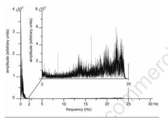
Figure 3. Complete spectrum and its high frequency (HF) part. Amplitude of HF component is for two orders of magnitude smaller than low frequency amplitude (example from Cačvina, Dec 10, 2011, 16:00 UTC).
