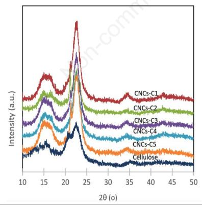
Figure 1. XRD of cellulose and CNCs are hydrolyzed with a reaction time of 1 to 5 hours.
