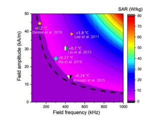
Figure 1. Whole-body SAR deposited in a 28 g mouse, as a function of the frequency and amplitude of the field (applied parallel to the body longitudinal axis). The maximum temperature increase is calculated for field parameters of pre-clinical studies (markers) exceeding Hergt-Dutz limit (dotted line).
