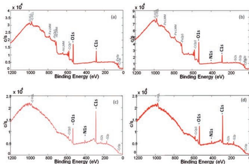
Figure 4. XPS spectra of: (a) SS plate; (b) SS-APTES plate; (c) SS-APTES-(PSS/PDDA)<sub>14</sub>; (d) SS-APTES-(PSS/PDDA)<sub>14</sub>-HE.
