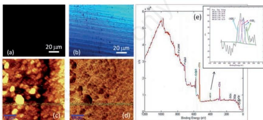
**Figure 1.** Fluorescence microscopy images of SS (a) and SS-APTES (b) plates. NC-AFM topographic (c) and phase (d) images of SS-APTES plates. (e) XPS spectrum and high resolution N1s spectrum of SS-APTES plates. Reproduced with permission from ref. 16. Copyright 2011, NSTI.
