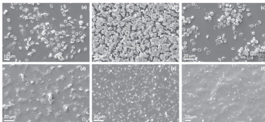
Figure 6. Scanning electronic microscopy (SEM) images of whole blood cells (a, b, c) on SS plates surface (a), SS-APTES surface (b) and APTES-(PSS/PDDA)<sub>14</sub>-HE surface (c). SEM images of human platelets (d, e, f) on SS plates surface (d), SS-APTES surface (e) and SS-APTES-(PSS/PDDA)<sub>14</sub>-HE surface (f).
