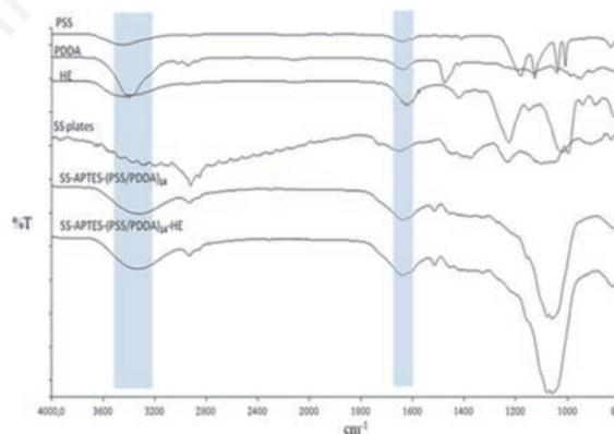
**Figure 3.** FTIR-ATR spectra of PSS, PDDA, HE, SS plates, SS-APTES-(PSS/PDDA)<sub>14</sub>, SS-APTES-(PSS/PDDA)<sub>14</sub>-HE.
