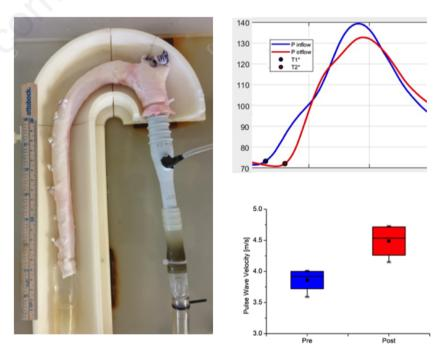
Figure 1. Left: Aortic sample in a 3D printed structure; Right: Experimental measurements of pressure during cardiac cycle (top) and pulse wave velocity (bottom).
